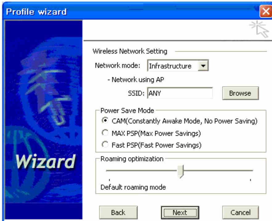
Select a "Network Mode" (Infrastructure or Ad-Hoc) and "SSID". You do not need to change the default settings of "Power Save Mode" and "Roaming Optimization" unless there is a special need to do so. Refer below for further explanation of each mode.
